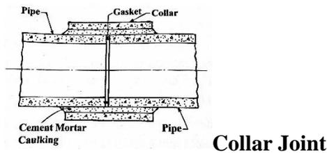
**Used for:** Cement concrete pipes.
