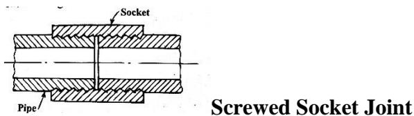
**Used for:** Galvanized iron pipes.
