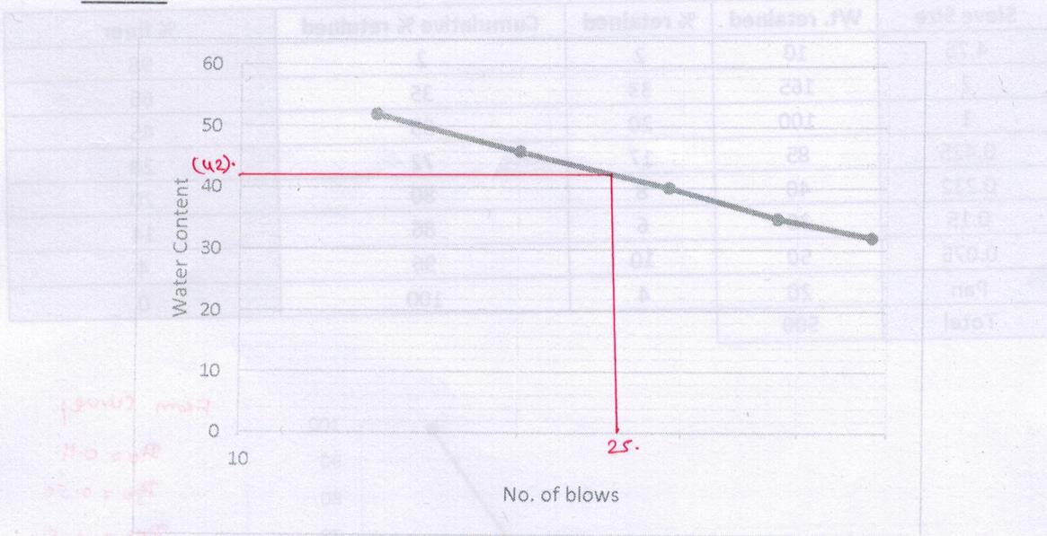
From the graph, the water content corresponding to 25 number of blows is 42 %, which is the required liquid limit for the soil.
