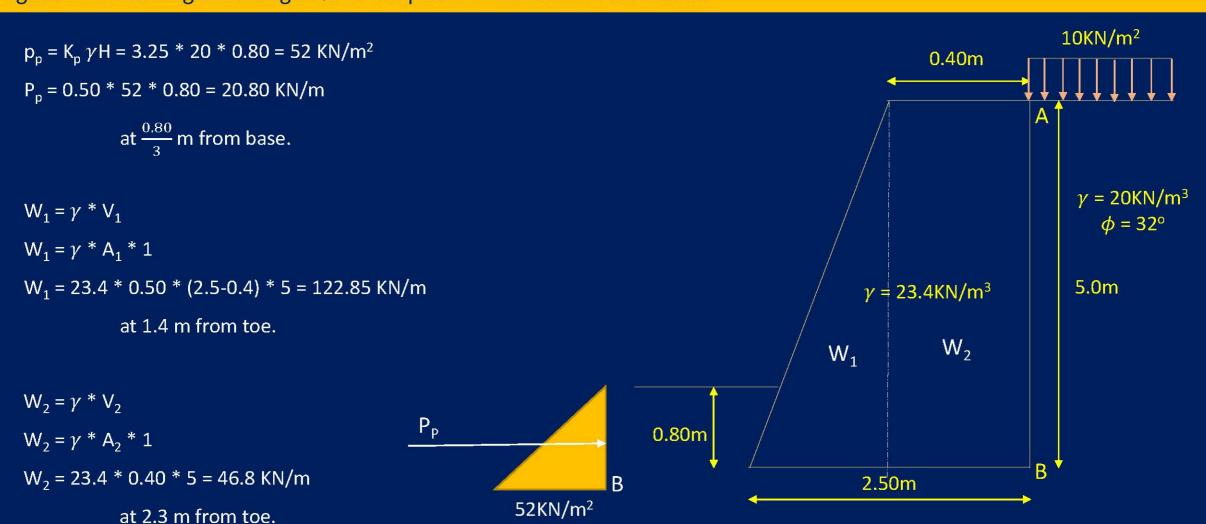
A masonry gravity wall as shown in figure is designed to support cohesionless soil. The unit weight of masonry wall is 23.4 KN/m<sup>3</sup>. The soil at the front and back of the wall is the same and have the same properties as given in figure. Calculate the FOS of wall against overturning assuming 50% of the passive resistance is mobilized.
