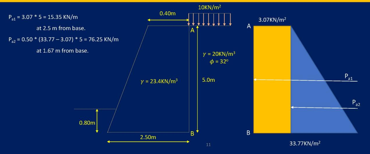
A masonry gravity wall as shown in figure is designed to support cohesionless soil. The unit weight of masonry wall is 23.4 KN/m<sup>3</sup>. The soil at the front and back of the wall is the same and have the same properties as given in figure. Calculate the FOS of wall against overturning assuming 50% of the passive resistance is mobilized.
