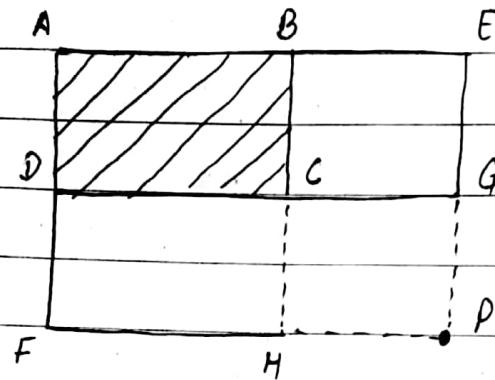
$$\sigma_v = q \left( I_{N_{AEPF}} - I_{N_{BEPH}} - I_{N_{DGPF}} + I_{N_{EGPH}} \right)$$
