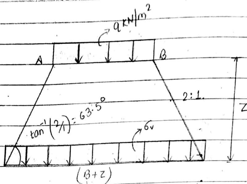
vertical stress ( $\sigma_v$ ) at a depth  $z$  below the soil surface under a different types of surface loading is given by,
