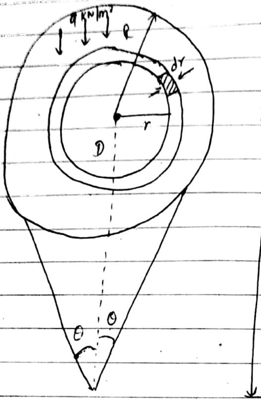
Let us consider a circular area of radius  $R$  carrying a uniformly distributed load of intensity  $q \text{ KN/m}^2$ . Consider an elementary ring of radius  $r$  and thickness  $dr$  of loaded area as shown. Let  $\theta$  be the apex angle at a depth  $z$ .
