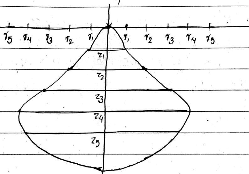
Procedure to draw an isobar diagram:-
