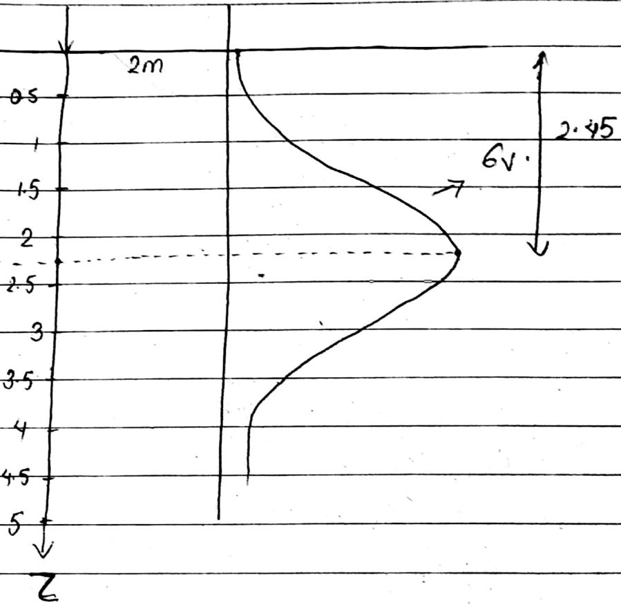
8.6 Vertical Stress distribution beneath the loaded area
