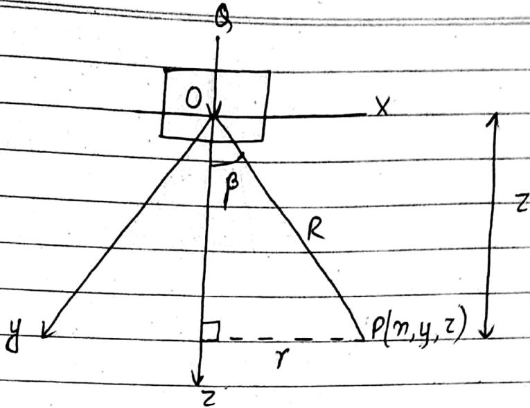
Let a vertical point load  $Q$  be acting at the soil surface at point  $O$ . Let  $P$  be the point in the soil mass having co-ordinates  $(n, y, z)$
