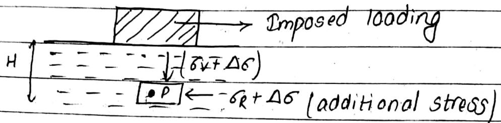
So, when a load is applied to the soil surface, the vertical stress within the soil mass increases. The vertical stresses at any point in a soil mass due to external vertical loadings are of great significance in the prediction of settlements of buildings, bridges, embankments etc.
